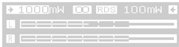
2. Use the 'UP' and 'DOWN' buttons to select the desired RF power output level.
