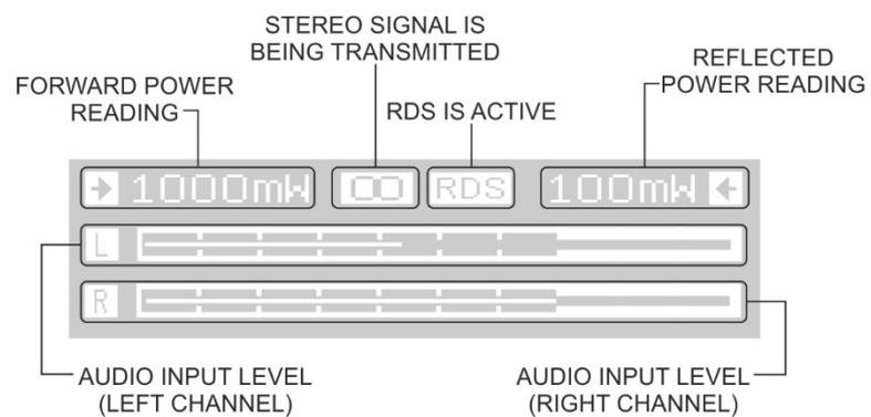
The front panel display shows the, forward power level (➡) reflected power level (⬅) audio input levels (ahead of any audio processing) and transmission frequency.
