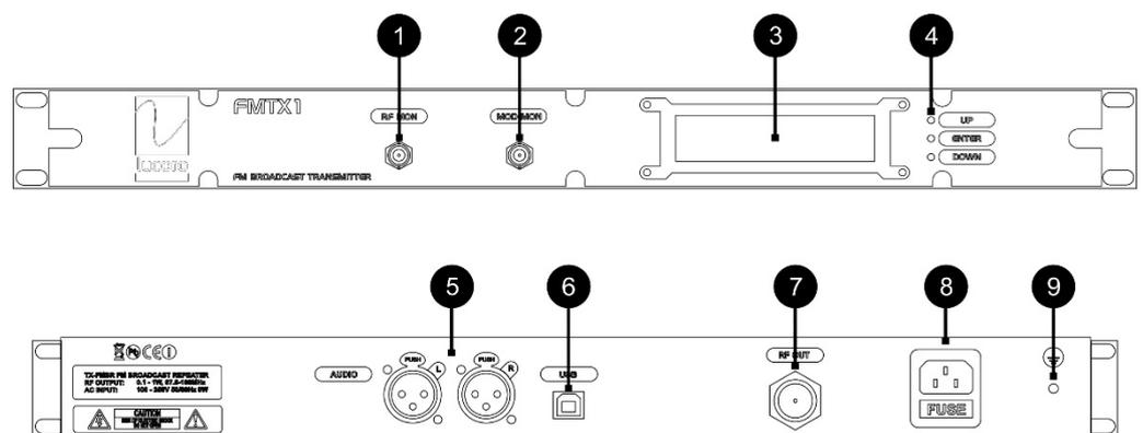
1. **RF MON** BNC connector for monitoring of the RF output. Output level will be the RF output level attenuated by approximately 40dB. Not to be used for measurement of harmonics.
