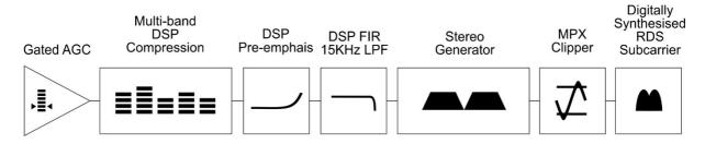
The processed stereo audio is then presented to the stereo generator circuitry, after which it is 'clipped' by distortion cancelling clipping algorithms, in order to keep the programme material to within the permitted deviation levels for FM transmission. This is the 'composite multiplex clipper'.
